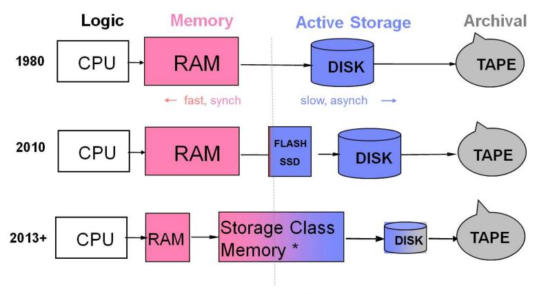
\* e.g. Phase change memory Memristor Solid Electrolyte Racetrack memory
