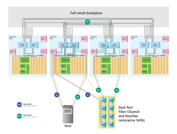
internal mapping mechanisms of physical hard drives and SSDs grant a very high granularity and efficiency in provisioning and space management. A proprietary Gen4 ASIC chip is devoted to manage and speed up all these operations, offloading the controller nodes CPUs and enhancing performance.
