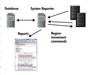
movements are controlled by a series of algorithms that weigh IOPS quantity, latency, and used space in the volumes involved to find the best match. Movements can be scheduled or automated while the system is running and without service disruption.
